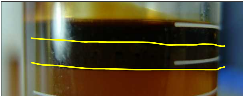
Figure 18 Result of gravity drainage flooding test with 2% of Surfactant
