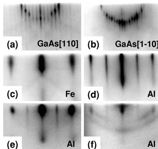
FIG. 1. 10 keV RHEED images along the GaAs  $\langle 110 \rangle$  directions of (a),(b) the initial (4 × 6) GaAs(001) surface; (c) a 0.9 nm Fe layer; (d) a typical Al overlayer grown on a continuous and fully crystallized ( $>0.5$  nm) Fe layer; and (e),(f) Al overlayers grown on 0.5 and 0.3 nm Fe layers, respectively, showing the mixed epitaxial and polycrystalline diffraction.
