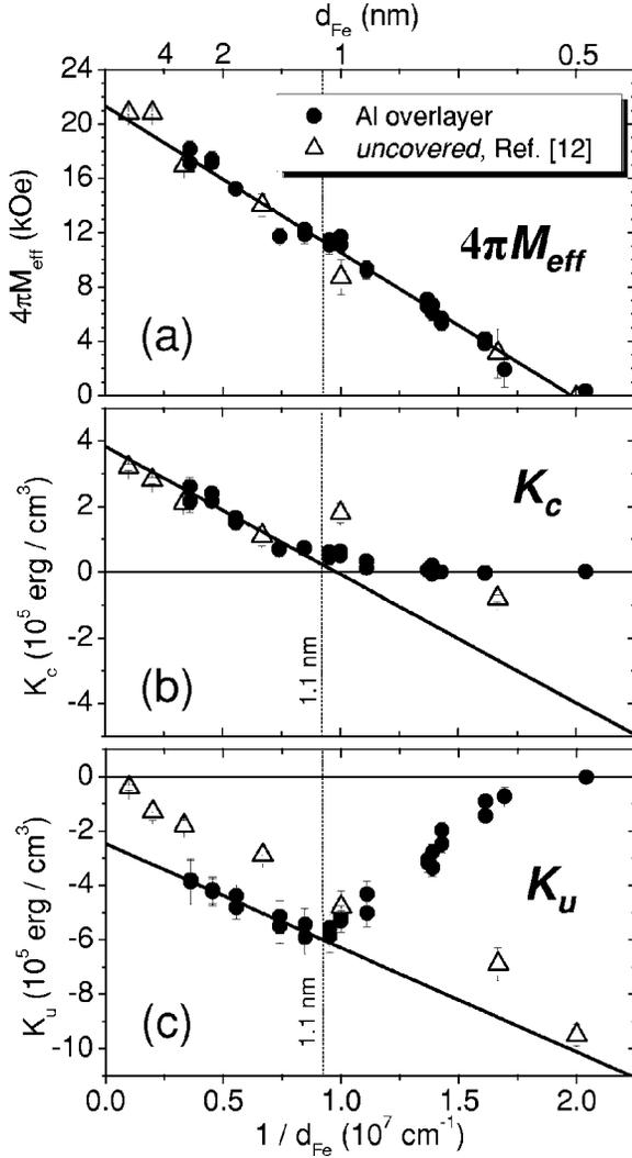
FIG. 3. Plots of our measured values of (a)  $M_{eff}$ , (b)  $K_c$ , and (c)  $K_u$  versus inverse thickness. Regression lines were fitted through the  $K_c$  and  $K_u$  data above 1.1 nm. For comparison, uncovered Fe data taken from Ref. 12 are included in the plot as the open points ( $\Delta$ ).
