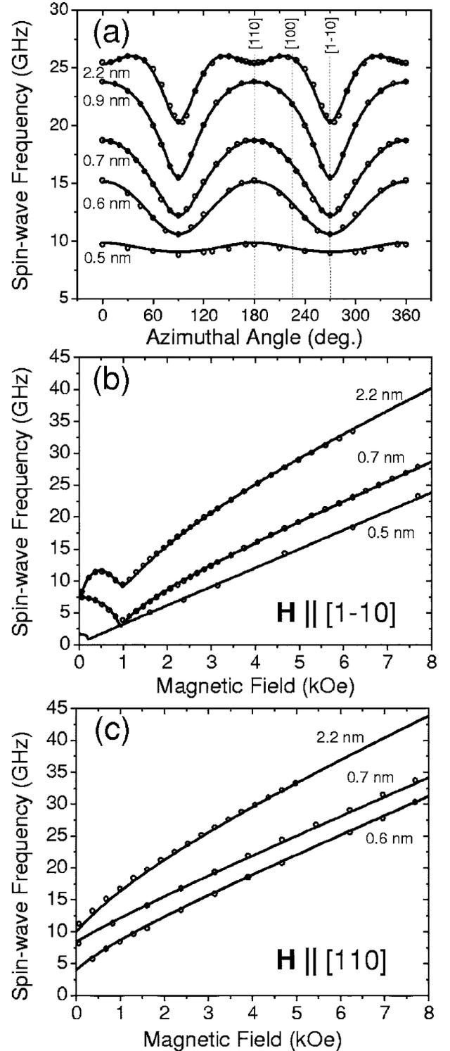
FIG. 2. BLS data (○) of the spin-wave frequency along with our fitted data (solid line) for (a) angular dependence at 3 kOe, and magnetic field dependence along the (b)  $[1\bar{1}0]$  and (c)  $[110]$  directions.
