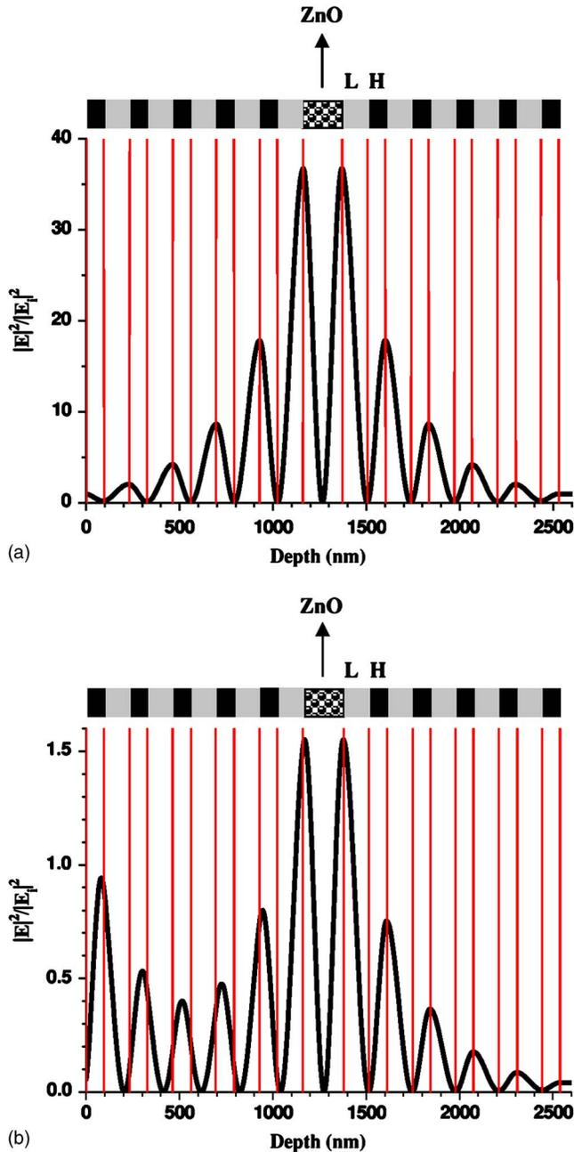
FIG. 3. (Color online) Spatial distribution of the squared field strength inside the ZnO-defect-containing photonic crystals: (a)  $(\text{Ta}_2\text{O}_5/\text{SiO}_2)^5/\text{ZnO}(210 \text{ nm})/(\text{SiO}_2/\text{Ta}_2\text{O}_5)^5$  (sample A), (b)  $(\text{Ta}_2\text{O}_5/\text{SiO}_2)^5/\text{ZnO}(219 \text{ nm})/(\text{SiO}_2/\text{Ta}_2\text{O}_5)^5$  (sample B). The incident wavelength was 800 nm.
