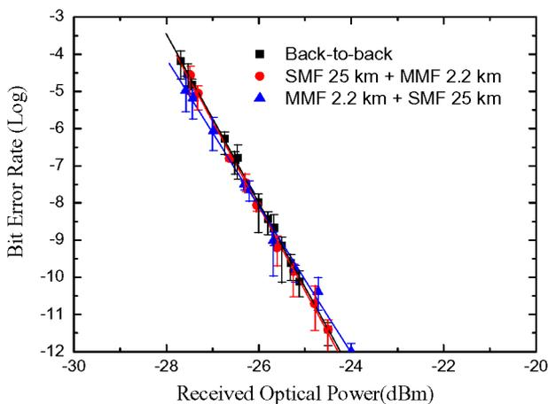
Fig. 5. Measured BERs for the hybrid SMF and MMF transmission.
