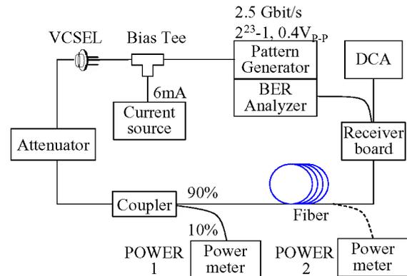
Fig. 1. Experimental scheme for the fiber transmission test of the 1.5- $\mu\text{m}$  VCSEL.
