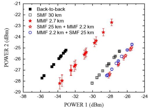
Fig. 3. Optical powers (POWER 2) measured after fiber transmission versus the input optical powers (POWER 1).
