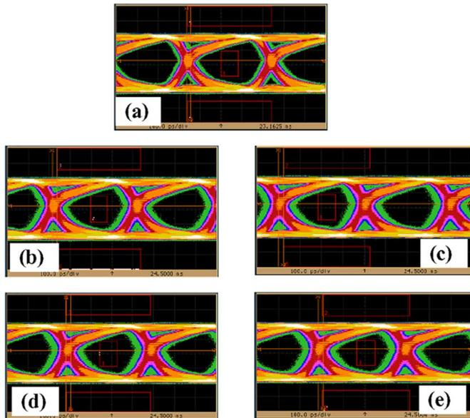
Fig. 2. Measured eye diagrams (a) BTB, (b) 2.7-km MMF, (c) 30-km SMF, (d) 25-km SMF + 2.2-km MMF, (e) 2.2-km MMF + 25-km SMF.
