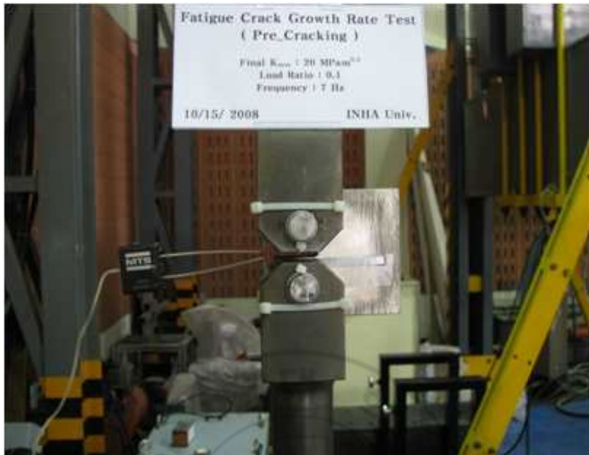
Fig. 12 Crack growth rate test at room temperature
